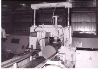
Figure 2. A close-up view of a saw cutting a wheel block.
