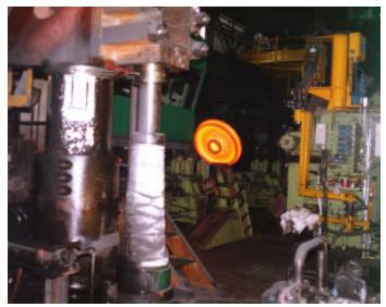
Figure 5. A robot manipulator passes a wheel from the rolling mill to the dishing and punching press. DISHING AND PUNCHING
