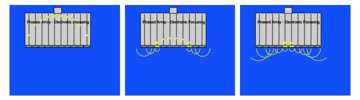
Figure 4. Wavefront focusing using phase delays.
