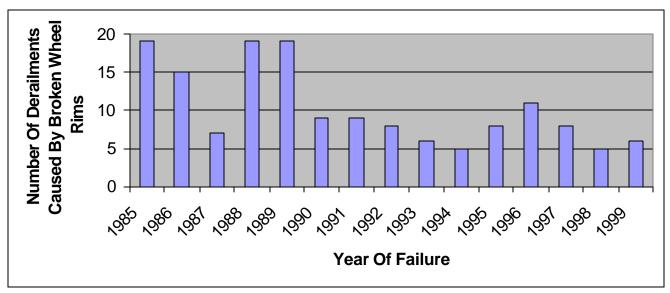
Figure 1. Number of broken wheel rims that caused derailments, 1985 – September 1999.
