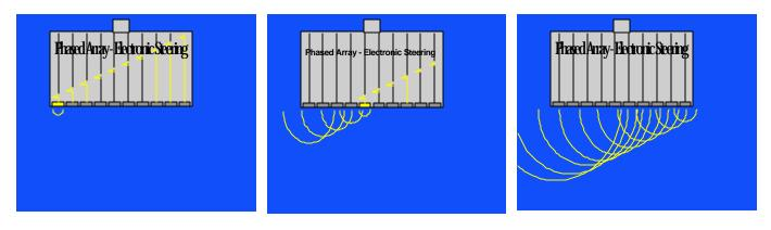
Figure 3. Wavefront steering using linear phase delays.
